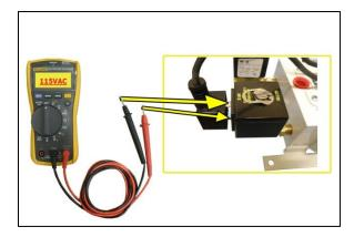
**8.4.5** Continue to measure for up to 90 seconds if no voltage is initially measured.
