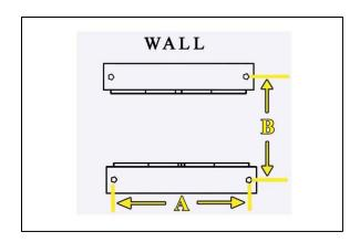
▲ IMPORTANT: When mounting, allow 2-1/2" above unit for tower removal and replacement.
