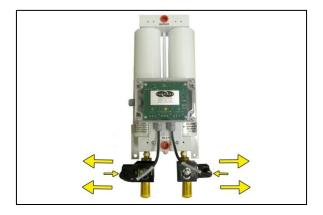
**8.4.4** Plug the HR back into the power source. While the unit is running, use a Voltmeter to measure the voltage across two terminals.
